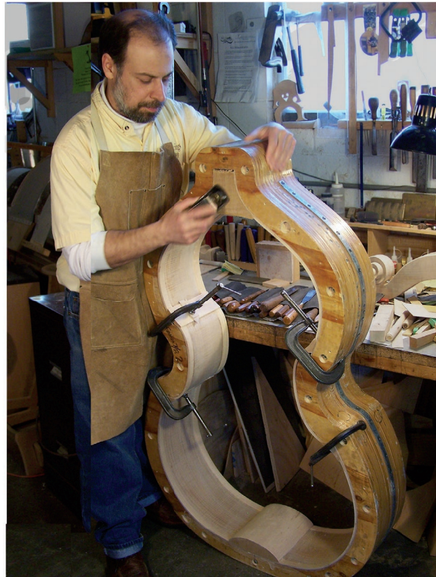
Planing down across the grain of the neck block in the mold.
